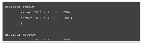
Here there are two load balancers defined. Default load balancing technique: **Round Robin** This block must be placed inside the http block.
